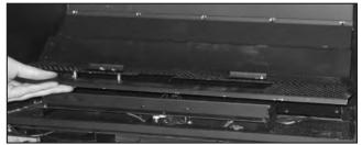
Figure 16: Removing Burner Tray.
